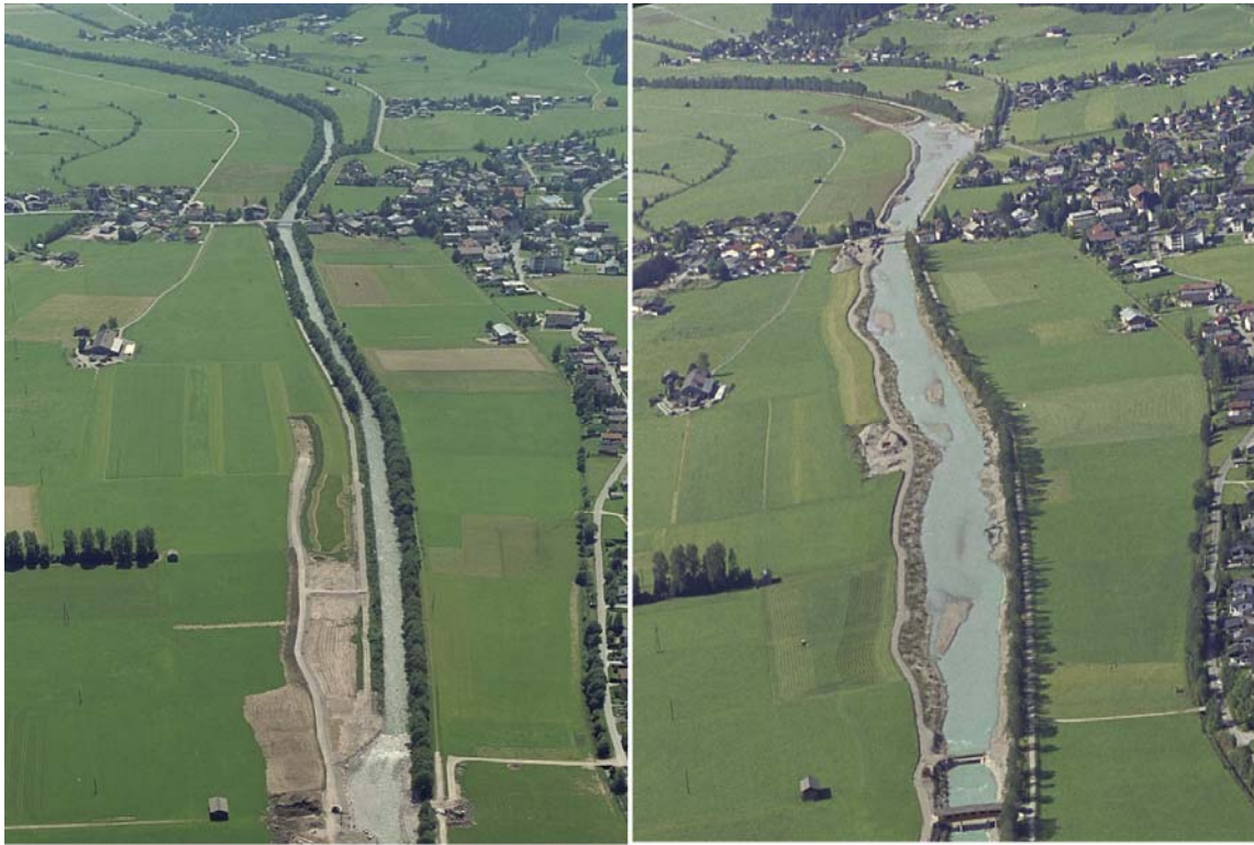
Fig. 20. and Fig. 21. The “Großache” a small river in the Tyrol. Widening up the river bed causes much more diversity and space for flood retention.
