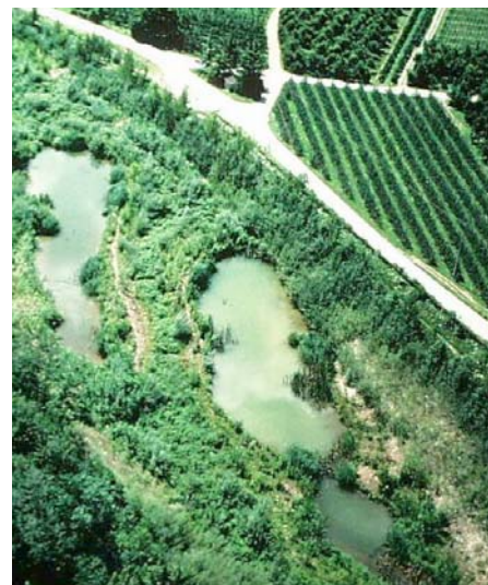
Fig. 18. and Fig. 19. Debris retention basin shortly after excavation and 5 years later. ( Southern Tyrol, Italy)
