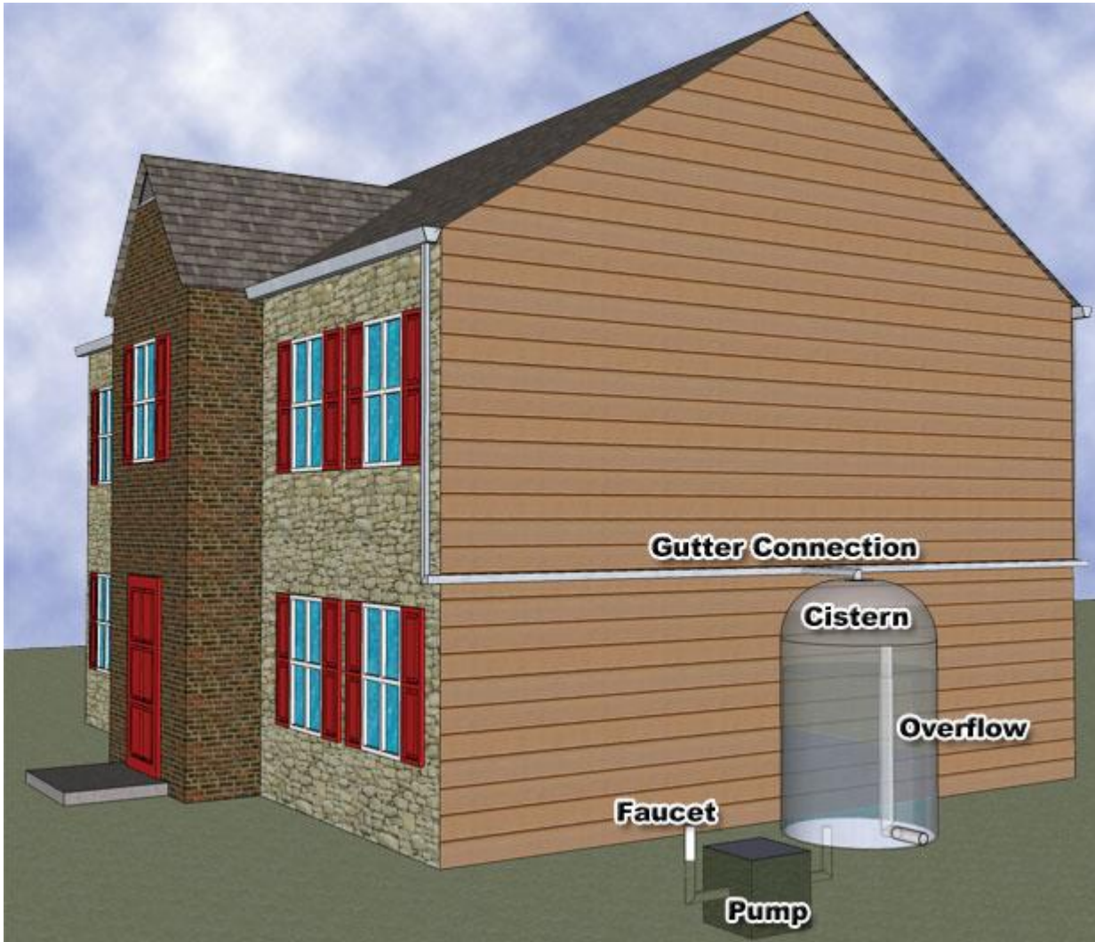
Basic rainwater harvesting system components
