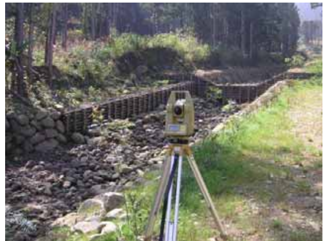
Figure 10. Monitor the displacement of wooden structure with laser theodolite at No.1 site
